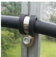
Place the 13mm semi-rigid pipe around the greenhouse and secure it to the bolts with the P-clips. It's intentionally a tight fit. If you're struggling to close the clips, you can remove the rubber lining - it's not strictly necessary but prevents the pipe from moving and flexing.
